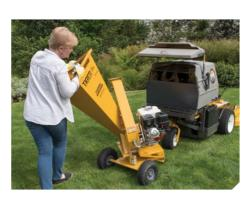
2) Lift the turntable locking pin and rotate the TIGER Chipper Shredder a quarter turn, and adjust the output chute height to the correct position.
