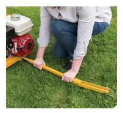
1) Insert spring loaded draw bar into guide on base.
