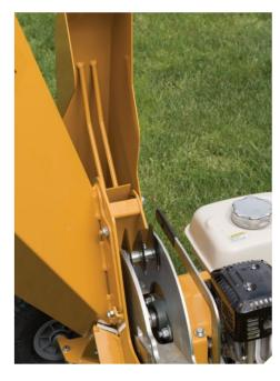
Two fixed gates hold garden waste in the cutting chamber, producing finer mulch for greater volume reduction and faster composting
