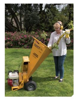
Two 80mm, offset blades chip branches up to 70mm in diameter, into smaller, manageable sizes for faster composting.
